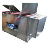
**24Hr Composting machine** recycles organic waste into a resource, organic fertilizer. The composting machine, **composts**, **sterilizes** and **dries** the organic fertilizer, thus readily available for farm use
