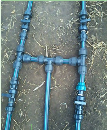
A system of main pipe joining a tee junction that distributes water to the sub main lines on both sides.
