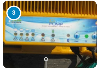
3 LED user interface: Allows to change between solar panel and battery mode, to monitor the performance of the pump and for on-site problem solving (indicates warnings and errors).
