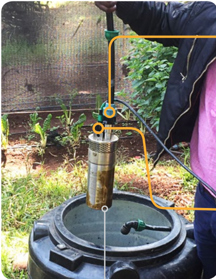
Pump placed or dipped into water source.
