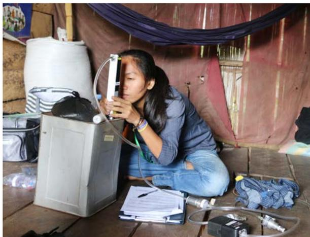
Figure 4. An enumerator testing the flow rate of an AirCheck XR500 pump, used for gravimetric sampling.
