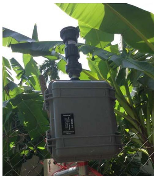
Figure 2. One of two AirMetrics MiniVol PM<sub>2.5</sub> samplers used to determine the influence of ambient air pollution on KAP and personal exposure.
