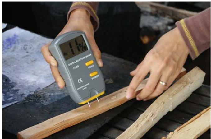
Figure 6. Wood moisture reading being taken for fuel use approximation calculations.
