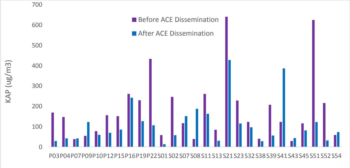
Figure 14. PM<sub>2.5</sub> kitchen air pollution (KAP) concentrations, shown on the y-axis, before (purple) and after (blue) ACE-1 stove dissemination for all of the 27 homes involved in the study with full 48-hour gravimetric exposure data and valid KAP measurements. Houheholds IDs are on the x-axis, those starting with 'P' represent Phnom Penh homes and those with 'S' are samlout homes.
