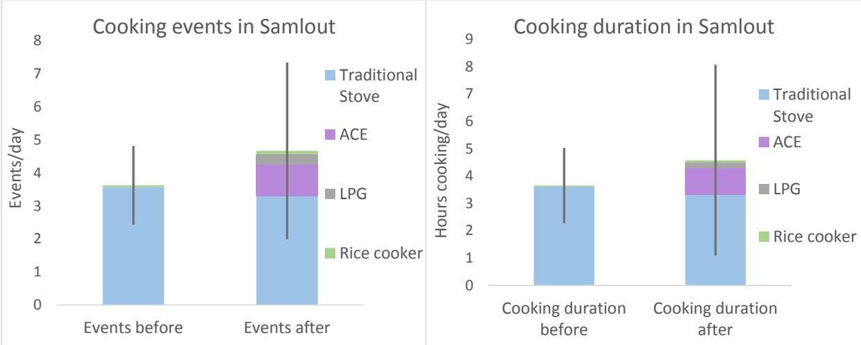
Figure 11. Stove usage and stacking, in terms of cooking events per day (left) and hours cooked per day (right), before and after ACE-1 stove introduction in Samlout. Error bars are  $\pm 1$  SD. Cooking events and duration of the respective cooking technologies are based on the entire participant pool (N=20), regardless of their ownership of the cooking technology.
