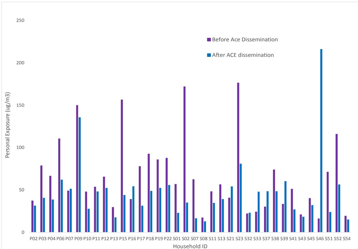
Figure 17. PM<sub>2.5</sub> personal exposure (PE) concentrations, shown on the y-axis, before (purple) and after (blue) ACE-1 stove dissemination for all of the 36 homes involved in the study with full 48-hour gravimetric exposure data measurements. Household IDs are on the x-axis, those starting with 'P' represent Phnom Penh homes and those with 'S' are samlout homes.
