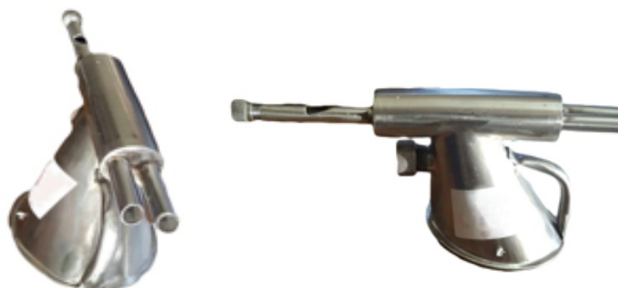
Figure 16 Alcohol gun (side and back view) for milk stability test
