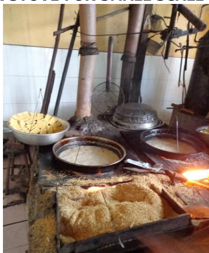
Picture 4: Soya cake making using the larger rice husk stove
