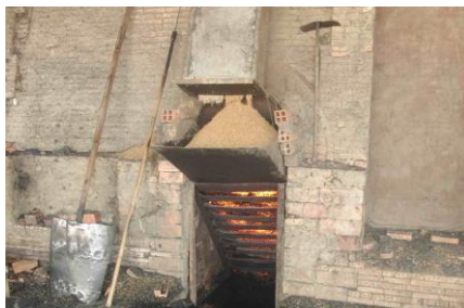
Picture 8: Brick kiln using rice husk as fuel
