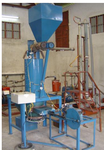
Picture 12: The 5-kW continuous gasification system coupled to a diesel engine
