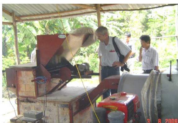
Picture 7: The automatic rice husk furnace for SRA-4 reversible flat-bed dryer
