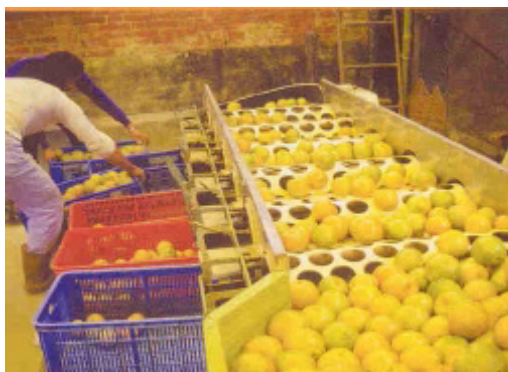
Figure 5.4 Mechanized grading of fruit by size, using different types of revolving drum
