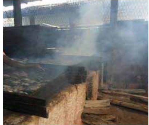
Figure 2: A lower-cost Chorkor Fish Smoker of mud construction.
