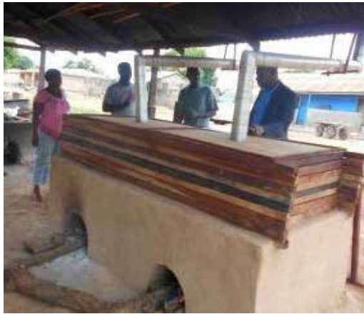
Figure 3: The Morrison Fish Smoking stove gives a 40% fuelwood saving over the existing Chorker stove.
