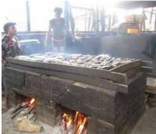
Figure 1: A Chorkor Fish Smoker (cement block) with fish being smoked on wire racks above a simple enclosed fire.
