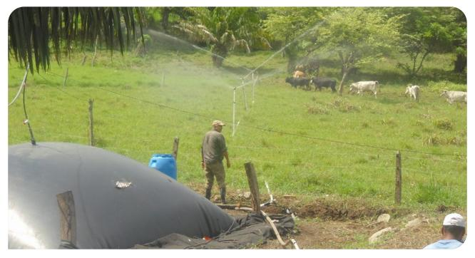
Productive use of biogas from a medium-scale biodigester for sprinkler irrigation in Nicaragua.
