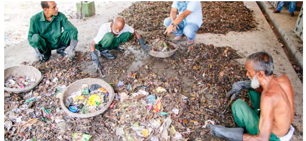
Kushtia FSTP workers removing rubbish from solid organic waste for co-composting purposes
