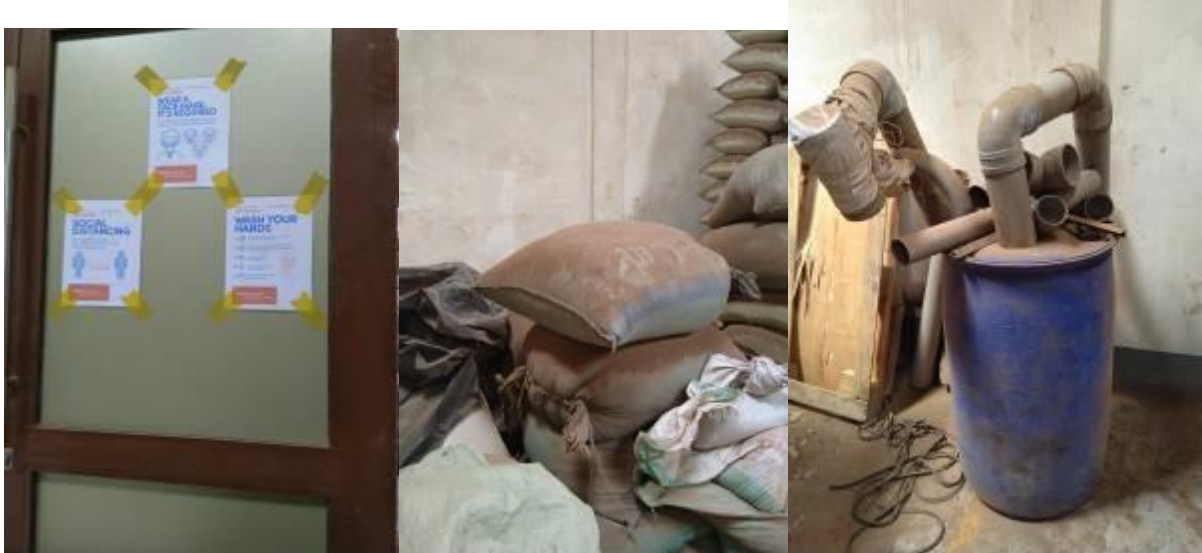
Figure 14: Signages (left); excessive dust on produce bag (centre); one of the tried dust remover (right)
