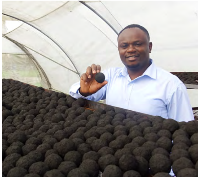
Round-shaped carbonised briquettes in drying beds
