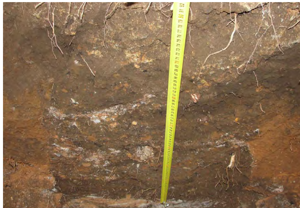
Decomposed sludge after 3.5 years at the Umlazi site in South Africa
