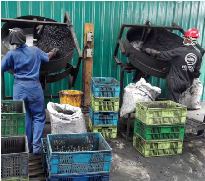
Agglomerator in operation using a rotating drum
