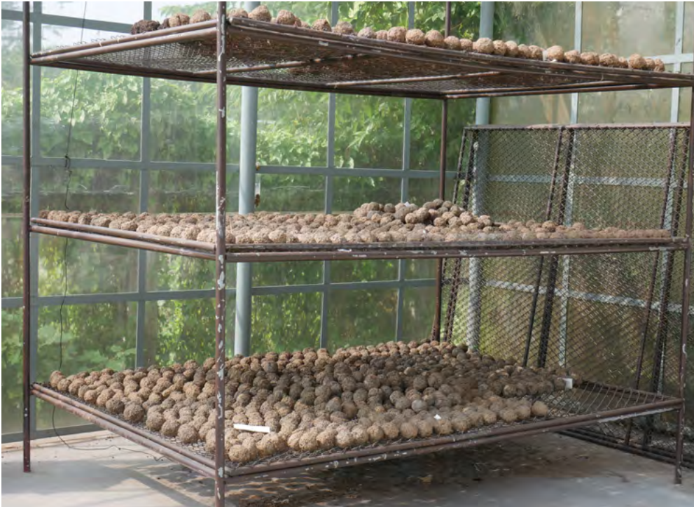
Briquettes on KCC drying racks/trays
